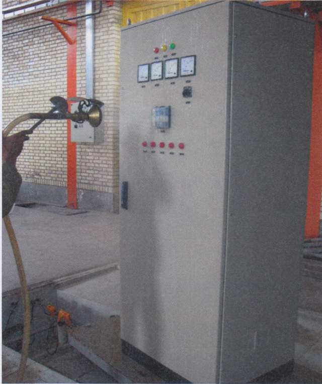
Figure 1; EUT under IPX4 test
