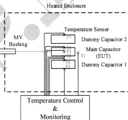
Figure 2: Sensors arrangement during the thermal stability test
